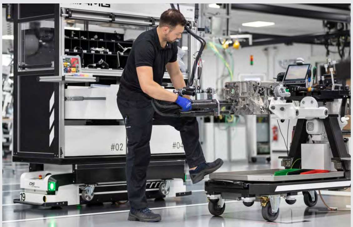
Assembly trolley and 'shopping basket' on an automated guided vehicles
