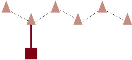
To eliminate daisy chains, approximately every third base station needs to be connected to the fixed network. Microwave backhaul capacity is then sufficient.
